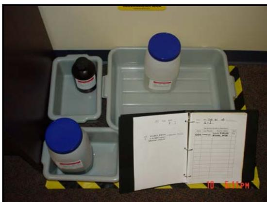
*Sample SAA set up with separate containment trays for incompatible chemicals*
